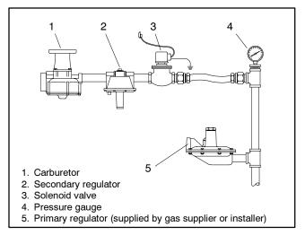
Figure 6-6 Typical LP Gas Vapor-Withdrawal System
